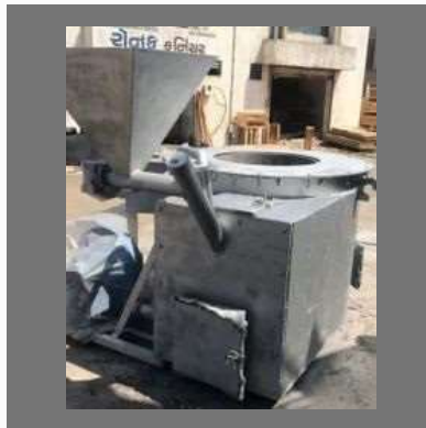
Bia Mass Aluminium scrap melting furnace
