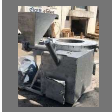
Aluminium Melting Furnace
